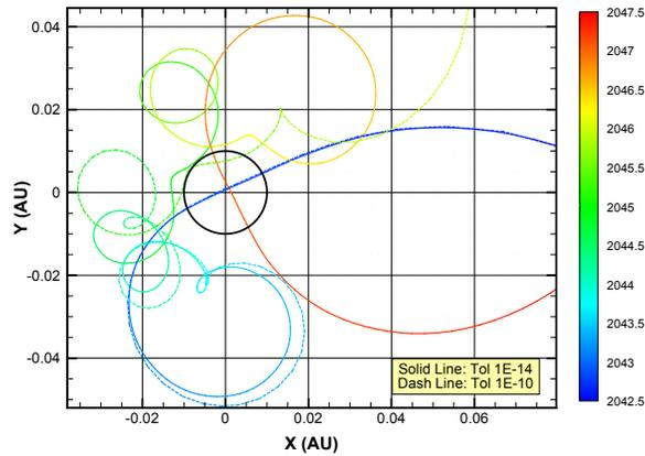
**Figure 5. Induced quasi-satellite motion of asteroid 1991VG in inertial axes. The trajectory propagation has been performed with two different numerical tolerances to check its robustness. Hill's sphere (dark) is added for comparison.**
