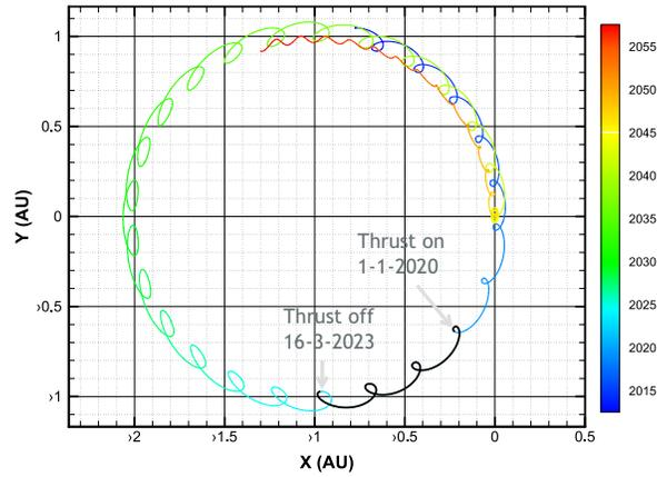
**Figure 3. Induced quasi-satellite motion of asteroid 1991VG in synodic axes.**
