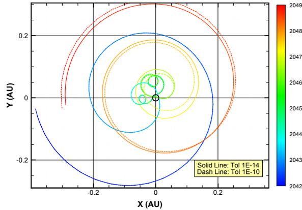
Figure 8. Induced quasi-satellite motion of asteroid 2010VQ<sub>98</sub> in inertial axes. The trajectory propagation has been performed with two different numerical tolerances to check its robustness.
