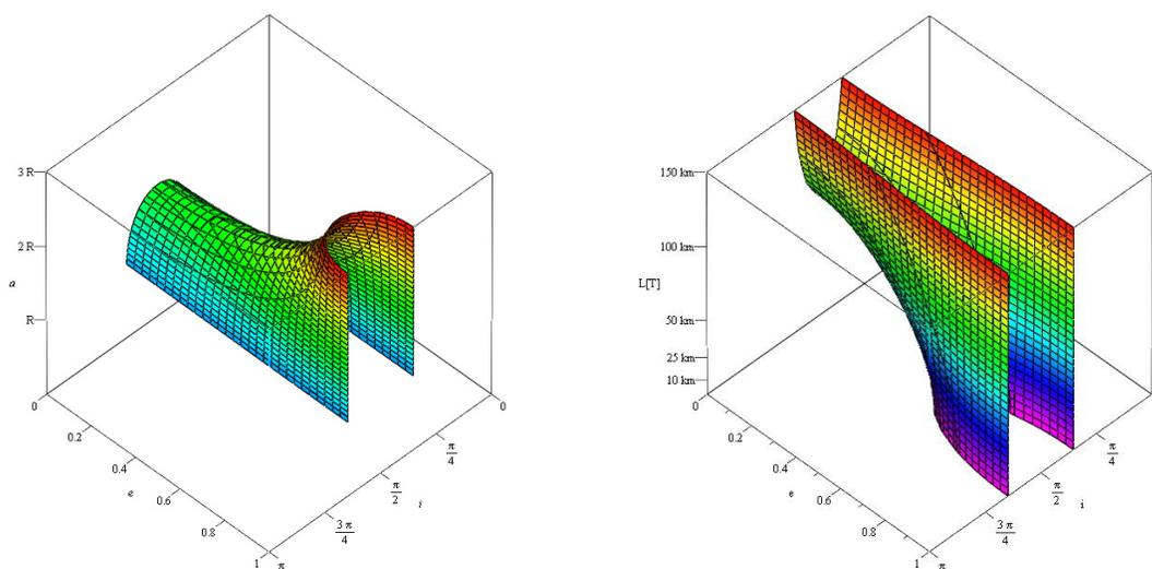
Figure 5: Locus of lunar frozen orbits that fulfil  $\omega = 0$ . **Left:** Fixed Tether Length **Right:** Fixed Semi-major axis.
