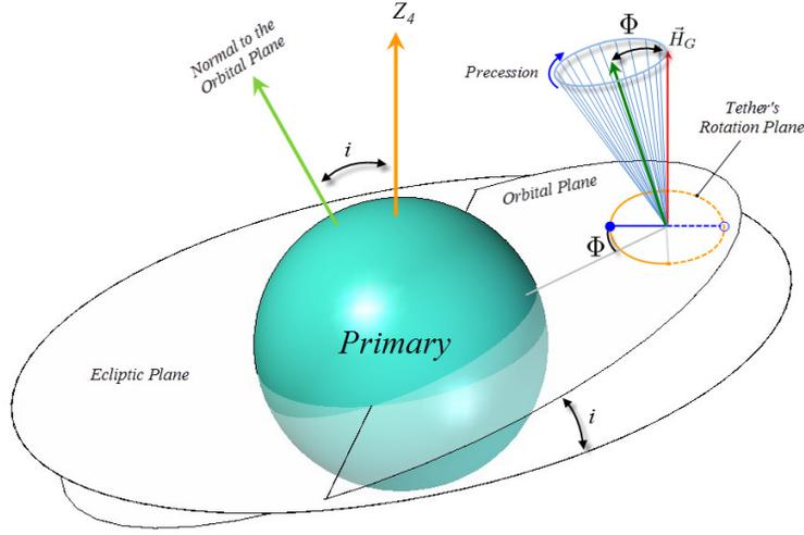
Figure 4: Scheme illustrating the precession of the tether's plane of rotation
