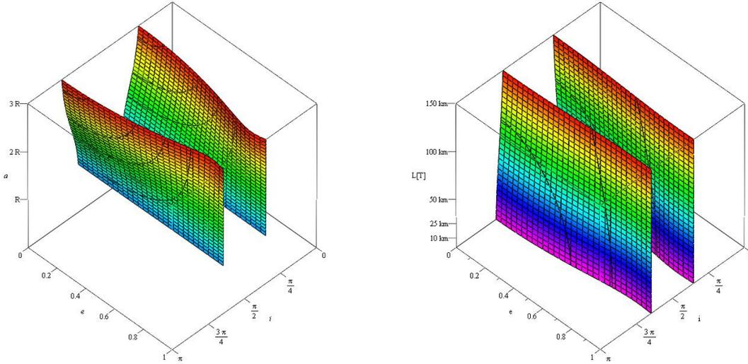
Figure 6: Locus of lunar frozen orbits that fulfil  $\omega = \pi/2$ . **Left:** Fixed Tether Length **Right:** Fixed Semi-major axis.
