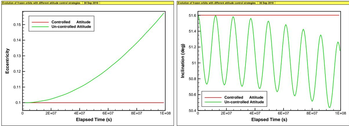
Figure 7: Evolution of a frozen orbit for different control strategies. The red line forces  $\phi_1 = \phi_2 = 0$  at any time, while the green line lets the tether’s rotation plane to precess. The simulation was carried for over 38 months. The nominal frozen orbit is:  $\omega = \pi/2$ ,  $e = 0.1$ ,  $a = 2R$ ,  $i = 51.601812^\circ$  and  $L_T = 40$  km.
