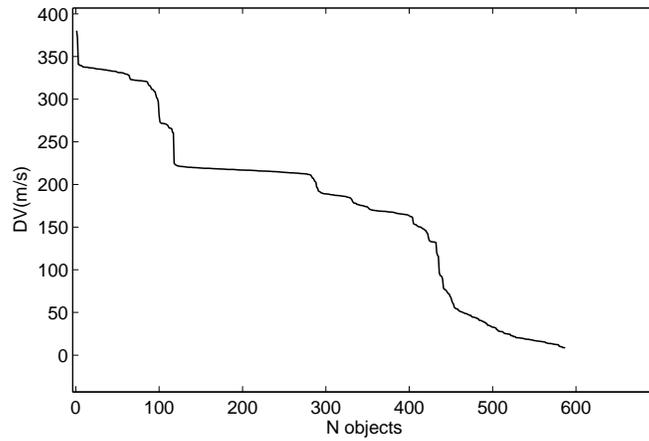
**Figure 3.  $\Delta V$  cost to lower the space debris perigee at 150 and 500 km altitudes with an impulsive apogee maneuver**
