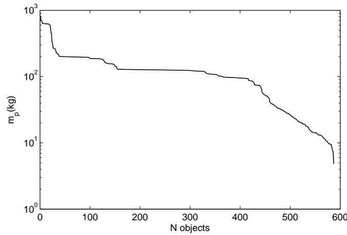
**Figure 4. Propellant mass cost to lower the space debris perigee at 150 km altitude with an impulsive apogee maneuver**
