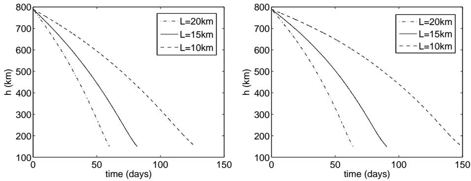
**Figure 7. Deorbiting curves for an H-2A 2nd-stage ( $m=4$  tons) starting from a circular 790-km-altitude 98-deg-inclination orbit, using a  $3\text{cm} \times 0.05\text{mm}$  tape electrodynamic tether of different length ( $L$ ) under maximum (left) and minimum (right) solar activity.**
