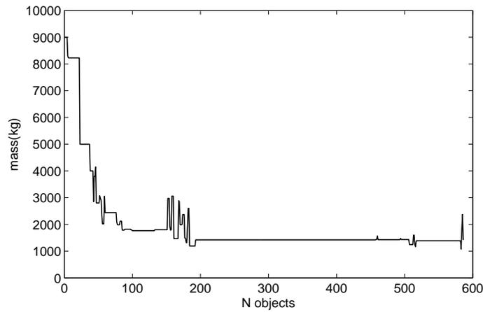
**Figure 2. mass of LEO spent upper stages ordered by descending hazard coefficient (Eq. 1)**
