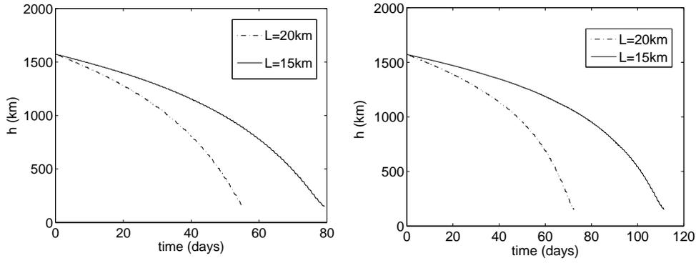
**Figure 8. Deorbiting curves for a Kosmos-3M 2nd-stage ( $m=1.4$  tons) starting from a circular 1572-km-altitude 74-deg-inclination orbit, using a  $3\text{cm} \times 0.05\text{mm}$  tape electrodynamic tether of different length ( $L$ ) under maximum (left) and minimum (right) solar activity.**
