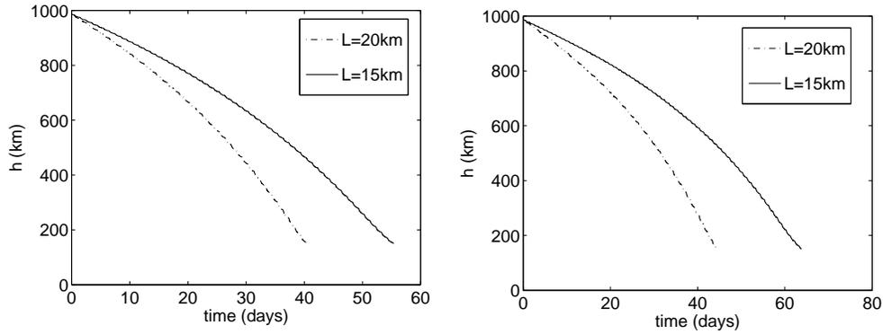
**Figure 9. Deorbiting curves for a Kosmos-3M 2nd-stage ( $m=1.4$  tons) starting from a circular 986-km-altitude 83-deg-inclination orbit, using a  $3\text{cm} \times 0.05\text{mm}$  tape electrodynamic tether of different length ( $L$ ) under maximum (left) and minimum (right) solar activity.**
