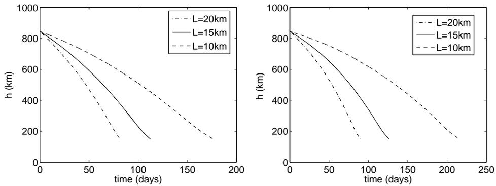
**Figure 6. Deorbiting curves for a Zenith 2nd-stage ( $m=9$  tons) starting from a circular 845-km-altitude 71-deg-inclination orbit, using a  $3\text{cm} \times 0.05\text{mm}$  tape electrodynamic tether of different length ( $L$ ) under maximum (left) and minimum (right) solar activity.**
