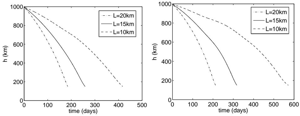
**Figure 5. Deorbiting curves for a Zenith 2nd-stage ( $m=9$  tons) starting from a circular 997-km-altitude 99-deg-inclination orbit, using a  $3\text{cm} \times 0.05\text{mm}$  tape electrodynamic tether of different length ( $L$ ) under maximum (left) and minimum (right) solar activity.**
