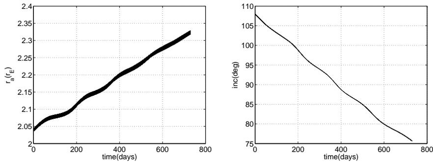
Figure 7: Semimajor axis and inclination variation for an optimally oriented passive EDT starting from a high inclination ( $i_0 = 108^\circ$ ) low Earth orbit ( $r_{p0} = 1.1r_E$ ) with initial eccentricity of 0.2. A 70 kg aluminum tape tether of 10 km length, 5 cm width and 0.05 mm thickness is employed. The payload mass is set to 100 kg.
