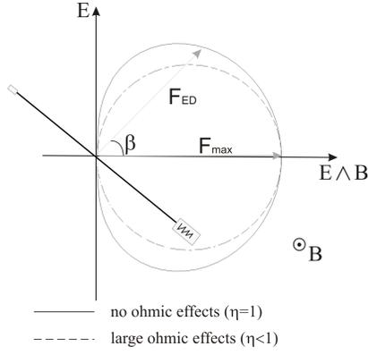
Figure 2: Force curve for a passive EDT as a function of the angle  $\beta$  between the tether line and the local motional electric field. The case of large and negligible ohmic effects are compared.
