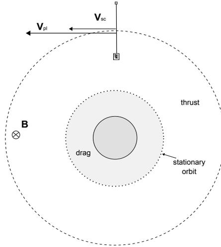
Figure 1: Thrust and drag conditions for an EDT in circular equatorial orbit around Jupiter
