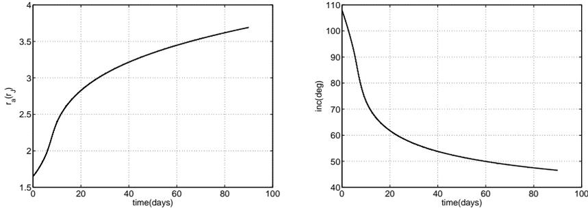
Figure 5: Semimajor axis and inclination variation for an optimally oriented passive EDT starting from a high inclination ( $i_0 = 108^\circ$ ) low jovian orbit ( $r_{p0} = 1.1r_J$ ) with initial eccentricity of 0.2. A 270 kg aluminum tape tether of 40 km length, 5 cm width and 0.05 mm thickness is employed. The payload mass is set to 200 kg.
