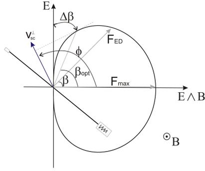
Figure 4: Force curve for a perfectly refelective solar sail as a function of the solar sail “clock angle”  $\beta$ .
