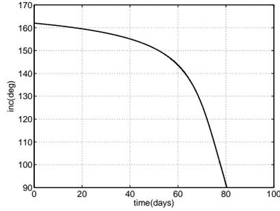
Figure 6: Inclination variation for an optimally oriented passive EDT starting from a quasi-equatorial retrograde low jovian orbit ( $r_{p0} = 1.1r_J$ ) with initial eccentricity of 0.2. A 270 kg aluminum tape tether of 40 km length, 5 cm width and 0.05 mm thickness is employed. The payload mass is set to 200 kg.
