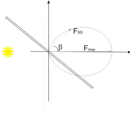
Figure 3: Force curve for a perfectly reflective solar sail as a function of the solar sail “clock angle”  $\beta$ .
